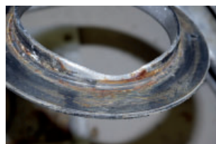
Wear of the flange ring
