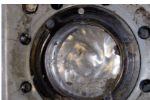
Wear of the slide plate
