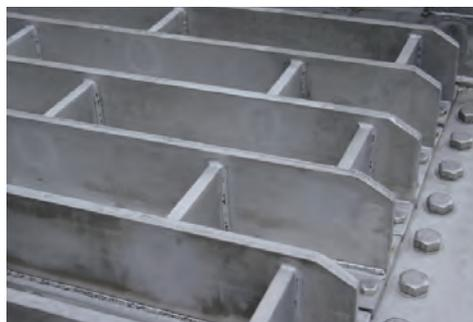
Only a inflexible shut-off valve is really stable and resistant against working pressure. We achieve this through the welded ribs to stiffen the housing.
