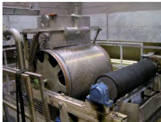
Double screening machine after optimisation
